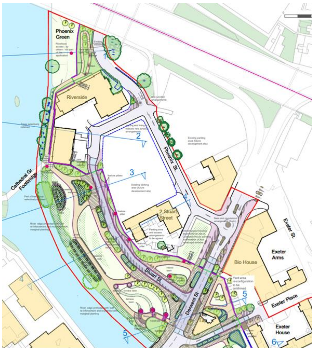
Figure 1: Proposed Flood Gate and Traffic Management Permanent Proposals for Derwent Street, Stuart Street, and Phoenix Street
