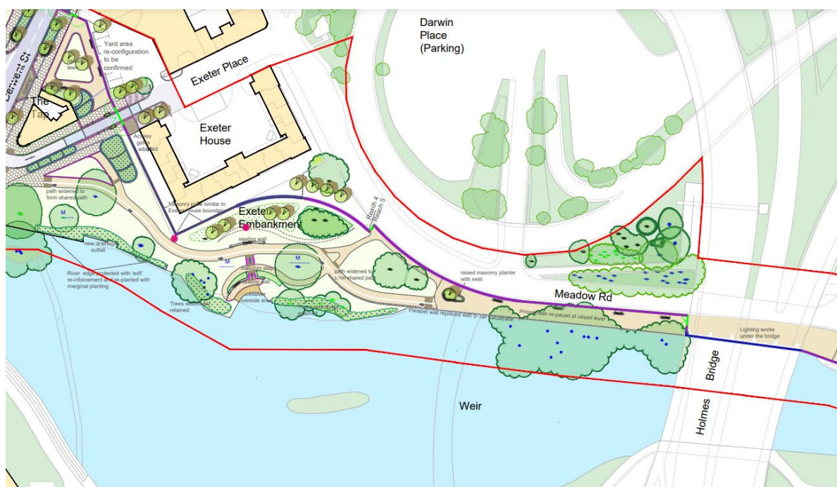
Figure 3: Proposed Flood Gate and Traffic Management proposals for Exeter Place and Riverside Cycle Path Adjacent to Meadow Road
