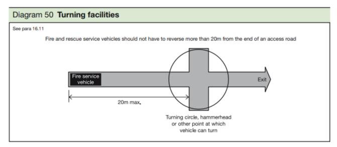
In this situation I would say that the fire tender would have to reverse part way up the drive, therefore the construction of the drive must be capable of achieving a load of 12.5 tonnes and be of a width of 3.7m
